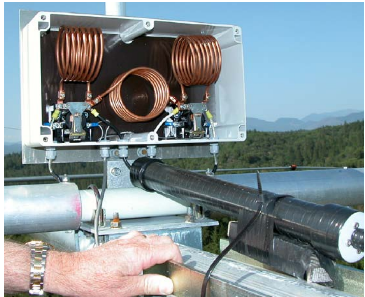
Fig 13-75 — K7ZV's driven element feed system. Relays add in loading inductors to switch from phone to CW band segments. The center coil is the hairpin matching inductor.
