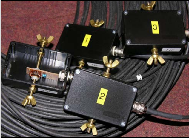
Fig 11-107 — Set of four identical RF current probes as described in Fig 11-106. Each transformer, along with its own cable (RG-58, about 25 meters long), was calibrated to be as identical as possible. The transformation loss varies between 32.5 dB on 160 meters and 32.8 dB on 80 meters.
