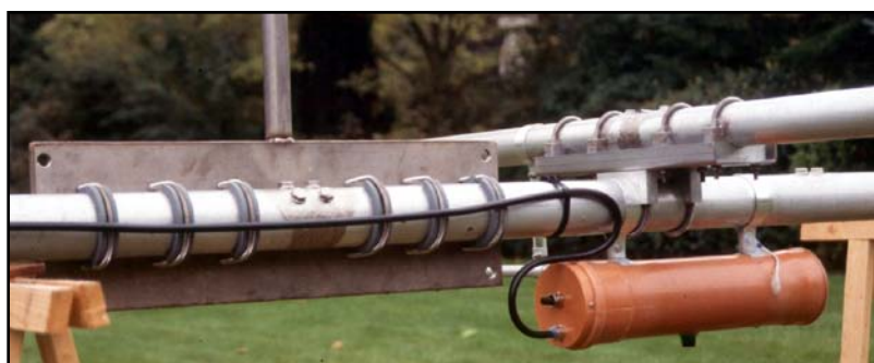
Fig 13-13 — The Omega matching system and plastic "drainpipe" box containing the two variable capacitors. Note also the boom-to-mast mounting plate made of 1-cm thick stainless steel. The boom is attached to this plate with eight U bolts and double saddles.
