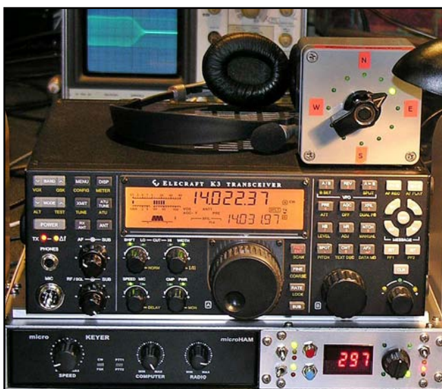
Fig 15-7 — The K3 at the “movable” operating position, on top of the homemade control box, which includes a Microham interface/keyer and the switching circuitry that makes it possible to do all the remote antenna switching and more.
