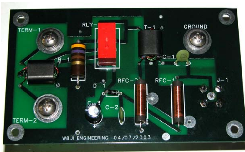
Fig 7-116 — This near-end receiving board, designed by W8JI, is used in the DX Engineering reversible antenna system model RBS-1P. It contains two transformers, a direction-switching relay and the termination resistor for the unused direction. In this configuration, only one direction can be used at a time.
