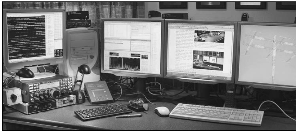
Fig 15-6 — On the left is the “movable” 2nd station at ON4UN, set up in the corner of the shack where ON4UN does his book writing and other PC related duties (2009 picture). Each of the K3s has its own PC and two screens. The screen on top of the K3 only displays CW skimmer (VE3NEA) and its call sign list. The larger screen to the right displays several N1MM contest software windows as well as a Power-SDR (IF) spectral display. Both displays are generated using LP-PAN with the Creative 0202 USB sound card, both sitting on top of the PC. The two screens on the right are connected to the “general applications” PC, on which the 5th edition of this book was created.
