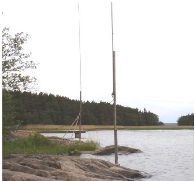
Fig 11-138 — Two-element 80 meter end-fire array at OH1NM, fed according to the opposite voltage feed system. This is not the shore of a lake, but the shore of the Baltic Sea.
