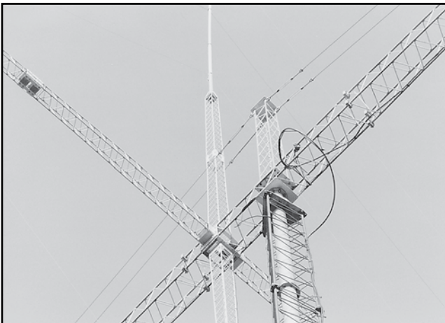
Fig 13-95 — This impressive 3-element full-size 80-meter quad, with an interlaced 5-element 40-meter quad, on a 26-meter (87-foot) long boom, sits on top of a self-supporting 30-meter (100-foot) tower at DJ4PT. The antenna was built by DJ6JC (SK).
