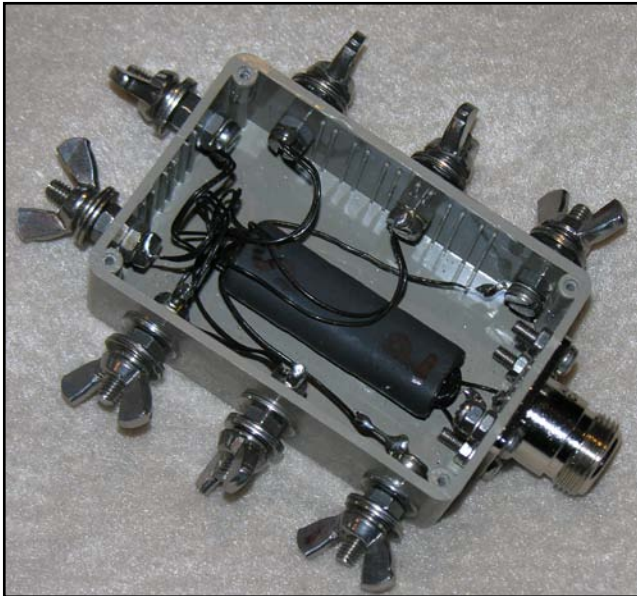
Fig 7-86 — A triple core multi-tap transformer yielding secondary impedances going from 200-612 \Omega for a 50- \Omega primary, or 300-920 \Omega for a 75- \Omega primary. This unit was specially built for determining the surge impedance of Beverage antennas.
