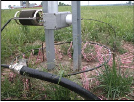
Fig 11-158 — Base of one of the elements of the K9DX Nine Circle. Note the high-Q loading coil and the ring (1 meter diameter) made of 10 mm copper, to which all of the 120 quarter-wave radials are connected.
