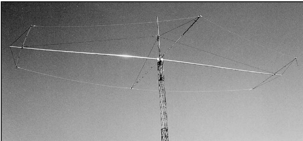
Fig 13-17 — The 3-element 40-meter NW3Z Yagi is mounted on a 21-meter crank-up tower at the Penn State University Dept of Electrical Engineering research facility at Rock Springs.
