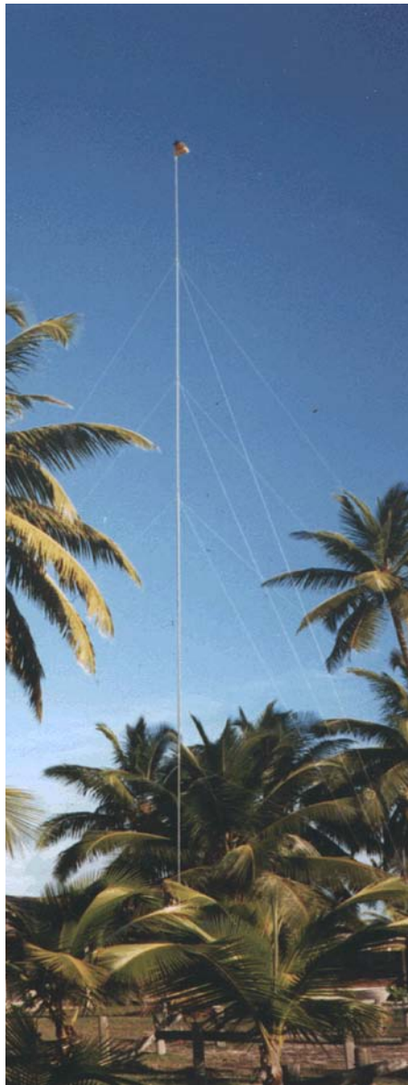
Fig 9-99 — The Titanex V160E antenna on the beach on VK9CR, surrounded by beautiful coconut trees. This 26.8-meter-long special DXpedition vertical weighs only 7.5 kg and disassembles into 2.1-meter long sections, ideal for traveling!
