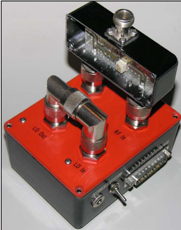
Fig 11-103 — The N2PK-designed VNA. The cover was removed from the impedance bridge. The two interconnected N connector are used for doing two port measurements (network analyzer mode).
