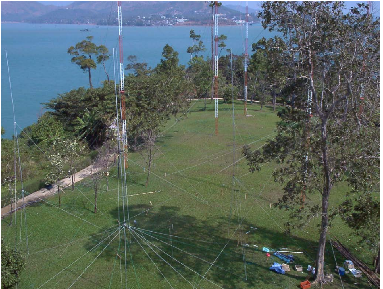
Fig 9-20 — XZ0A had an ideal location for far-field reflection efficiency: Saltwater all around. Four Squares were used on 80 and 160 meters, resulting in signals up to S9+20 dB in Europe on Top Band, quite extraordinary from that part of the world.
