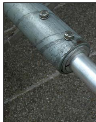
Fig 7-19 — Transition of the 60.3-mm OD steel pipe to the 35-mm OD aluminum element.
