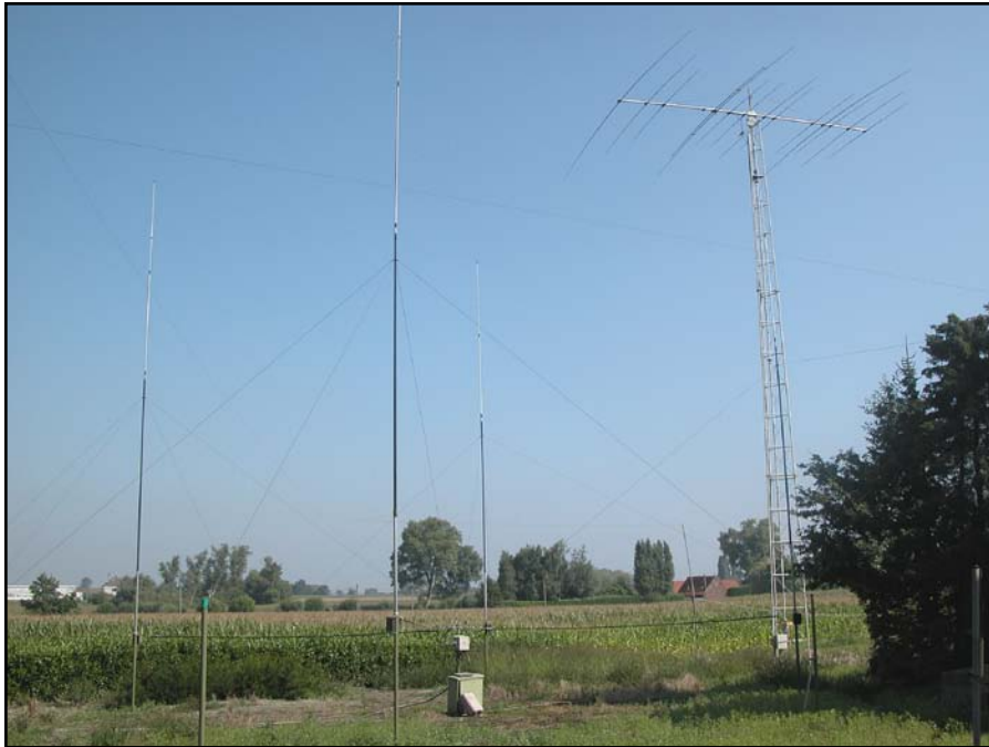
Fig 15-4 — Way in the back, almost 100 meters behind the house, are the two “multiplier” antennas — a Force 12 C31XR (excellent triband antenna!) and a 40-meter four square with elevated radial system.
