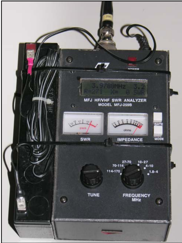
Fig 11-100 — I always use my MFJ-259B antenna analyzer outdoors with a small 12 V lead-acid battery strapped on its side, as I hate to run out of power in the field.
