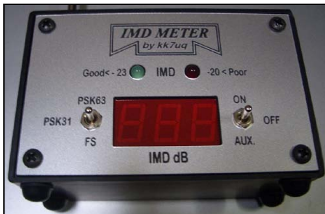
Fig 3-30 — KK7UQ developed an IMD meter to show PSK operators at all times how much transmitter IMD products are down. This is what we need for SSB transmitters!
