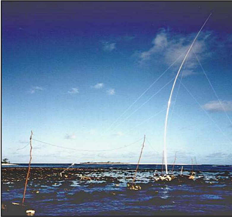
Fig 9-41 — The Titanex V160E antenna on the beach at 3B7RF (St Brandon Island). Note the two elevated radials about 2 meters above saltwater. The combination of one or two elevated radials with a perfect ground underneath is hard to beat.
