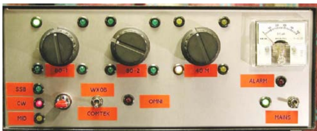
Fig 11-172 — Array-direction switch box at ON4UN, with a Four Square direction switch for 40 meters and two switches for 80 meters. A switch selects the Comtek or another feed system (at this time the optimized hybrid feed system is being tested alongside). Relative power and alarm circuit (Fig 11-173) is measuring the power in the dummy load. The lever switch on the left selects one of three band segments on 80 meters.
