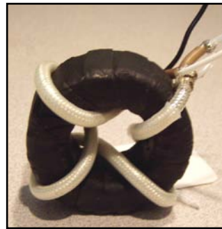
Fig 11-163 — A 9:1 transformer made by John, K9DX. The transformer counts 4 trifilar turns. The trifilar wiring is made by using a small Teflon coax equipped with a second shield. See text for details.
