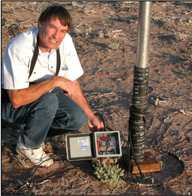
Fig 7-68 — K7CA at the base of one of the array elements. Note the heavy copper ring to which all 120 radials are soldered. The two loading coils are wound on the black insulator, while the relay and the 1:4 transformer are placed in a plastic enclosure.
