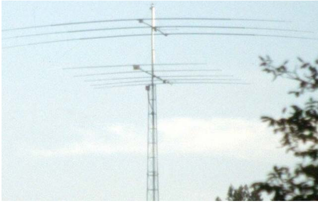
Fig 13-5 — No, this is not a 15-meter Yagi on top of a 6-meter Yagi, as you might judge from the very small degree of sag in the elements, but the 3-element 40-meter Yagi at ON4UN. The antenna is 30 meters high, 5 meters above a 20-meter Yagi (15-meter boom). The amount of sag in an element is a very good indicator of the mechanical strength (read: wind resistance) of the element.
