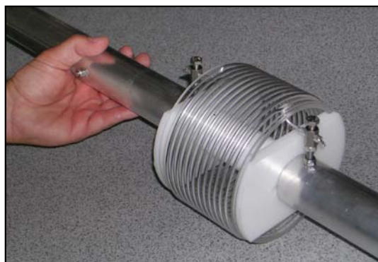
Fig 13-38 — Loading coil as manufactured by Optibeam and used in their 2- and 3-element reduced size Yagis.
