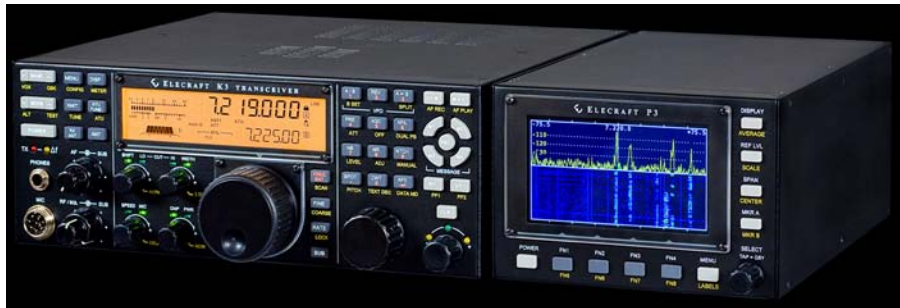
Fig 3-14 — The ever-so-popular Elecraft K3 with its own optional spectral and waterfall display (the P3). You can control a lot of functions of the K3 from the P3.
