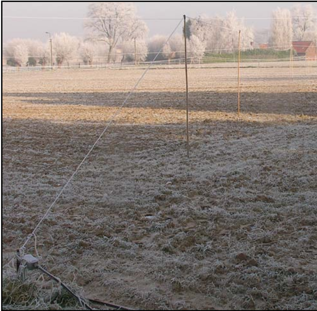
Fig 7-104 — Sloping end section of the 300 meter long Beverage in the direction of Japan at ON4UN. The sloping section is approximately 15 meters long.
