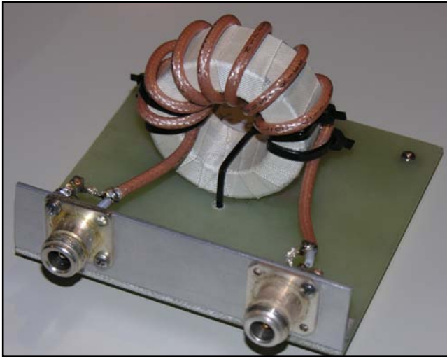
Fig 11-38 — The 180° flipped coax phase reversal transformer, after a design by K9DX. This unit for 80 meters uses 8 turns of RG-303 on a stack of two FT-250-61 (61 mix) cores.
