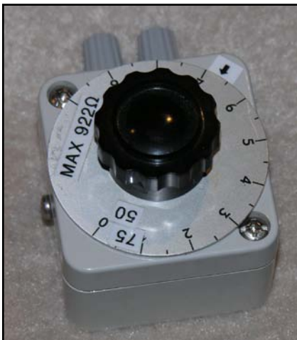
Fig 7-87 — A high-quality, linear 1-k \Omega potentiometer is a valuable instrument for testing Beverages and Beverage transformers.
