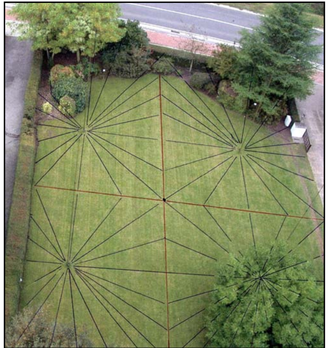
Fig 7-42 — Radial layout used at ON4UN's mini Four Square. Each vertical has 18 short ground radials, which are soldered to a bus wire. A 1.5-meter long ground rod is used at each element.
