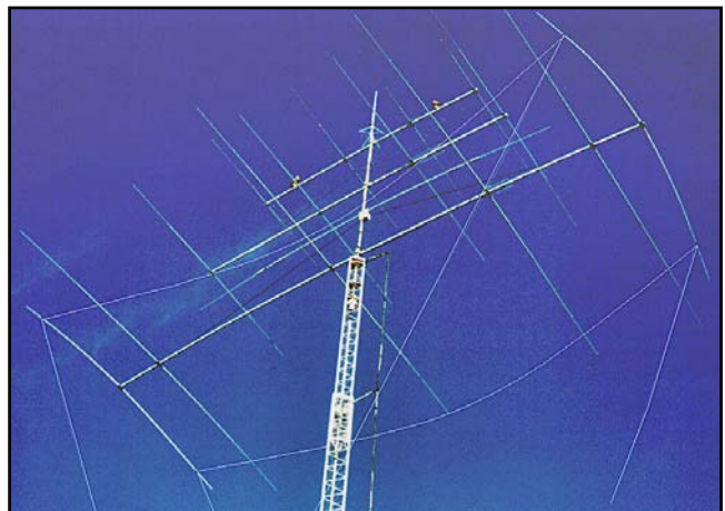
Fig 13-95 — This impressive 3-element full-size 80-meter quad, with an interlaced 5-element 40-meter quad, on a 26-meter (87-foot) long boom, sits on top of a self-supporting 30-meter (100-foot) tower at DJ4PT. The antenna was built by DJ6JC (SK).
