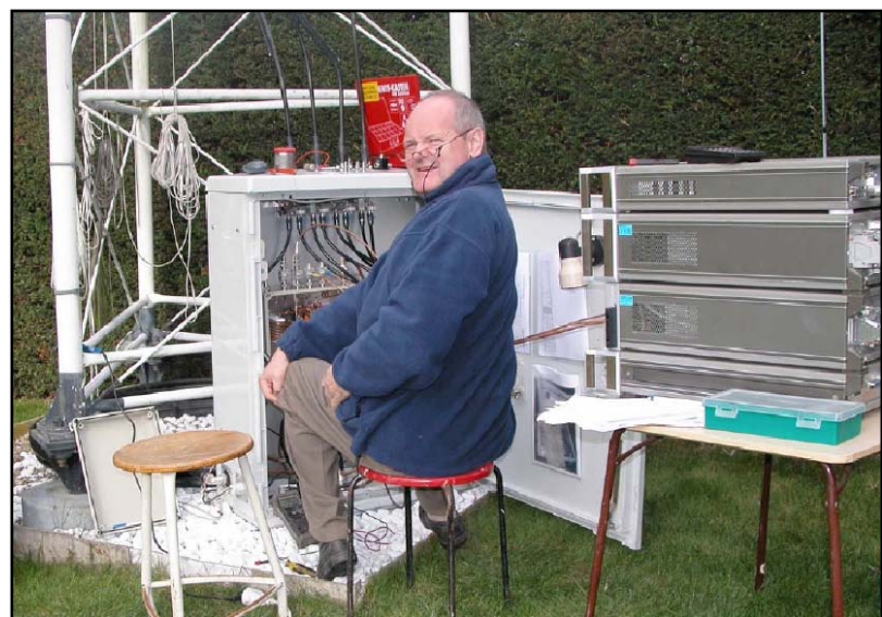
Fig 9-76 — Roger Vermet, ON6WU, with his professional antenna measuring setup, tuning the new vertical at ON4UN. An HP network analyzer is used which directly produces a Smith Chart. Although such sophisticated test equipment is not necessary to tune a vertical, it is very instructive to know the impedance (admittance) curve.
