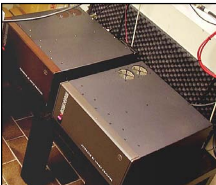
Fig 15-11 — At ON4UN the two ACOM 2000A amplifiers are located in a small room next to the shack, in order to keep all the heat (cooling heat) and noise out of the shack. You really don't have to do it for the noise as these units are actually quieter than many PCs.
