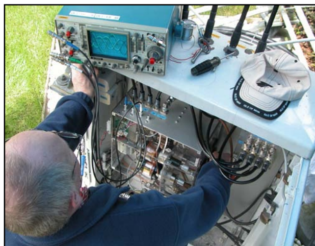
Fig 11-174 — Roger, ON4WU, tuning the Lewallen/Lahlum feed system using a five channel scope. The box uses four vacuum variables, two of them in series with a coil, making the combination a variable coil. Note the overlay (generated on the computer on the scope screen, showing the amplitude and phase of the three different signals (see also Fig 11-98).
