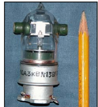
Fig 11-150 — Russian-made small vacuum relays with a single make/break contact are ideally suited for a relay matrix.
