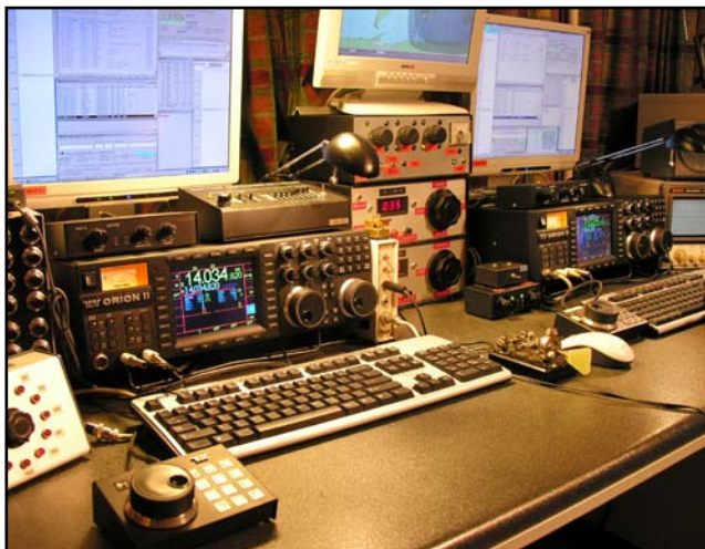
Fig 15-5 — SO2R setup at ON4UN using two Orion II transceivers (2005). On the extreme left of the picture we see the 12 position rotary switch for selecting the Beverage antennas.
