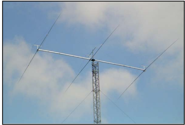
Fig 13-98 — The Optibeam OB3-80, a 3-element high-Q coil loaded Yagi.
