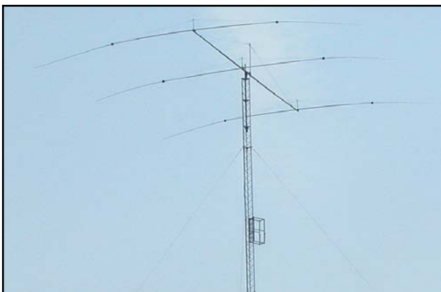
Fig 13-33 — Three-element 80-meter Yagi using shortened elements at W6KW. The Yagi uses the high-Q loading coils developed by W6ANR. See text for details. The 55-meter high antenna sits on a knoll surrounded by flat terrain. To work on the antenna the platform visible along the tower is unfolded, and the Yagi is tilted 90° so that the center of the element is easily accessible from the platform.
