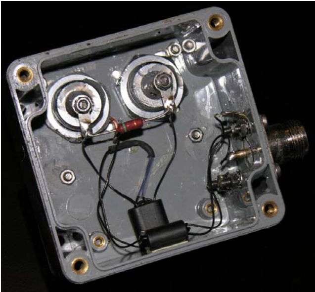
Fig 7-133 — Combiner box for the 2-element end-fire array at ON4UN.
