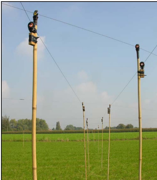
Fig 7-110 — This shot taken on the author's Beverage field shows two parallel running Beverages (receiving from opposite directions) and a Beverage crossing. See text for details.
