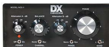
Fig 7-71 — W8JI developed the NCC-1 noise canceller/phase controller, which is available from DX Engineering.
