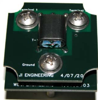
Fig 7-117 — The far end reflecting transformer with its three terminals: two going to the two-wire Beverage and one going to ground (part of the RBS-1P system).
