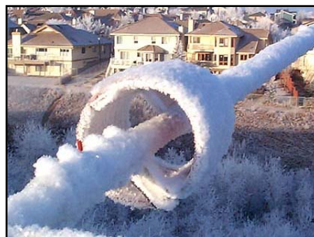
Fig 13-36 — It is obvious that unprotected coils can get severely detuned by ice loading as shown in this photo at VE6WZ.
