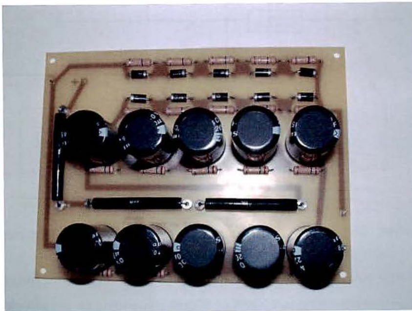
3600 volt power supply Board
