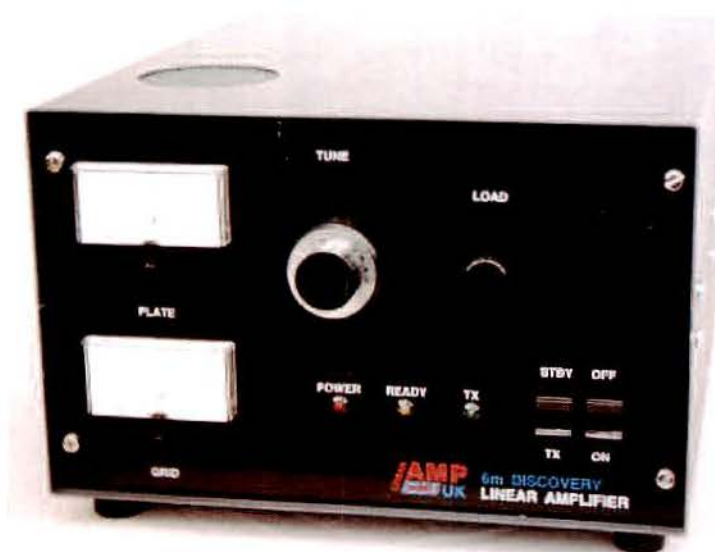
Front panel of the 6 metre 3CX800A7 amplifier
