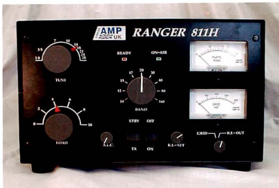
Front Panel layout of the 811 amplifier
