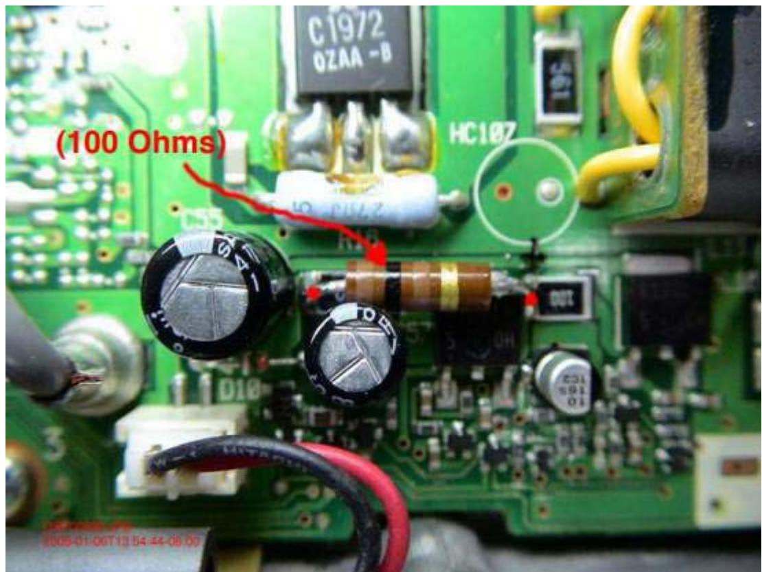
Above: As you can see, I tack-soldered the resistor to the two lands indicated by the RED DOTS. I evaluated the fan's noise with the covers off; In retrospect, I would
