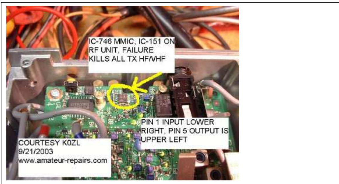
uPD1678, icom number is 1110001890, lists about 10 bucks or less. Changing this chip requires proficiency in surface mount desoldering, and anti-static protection measures.
