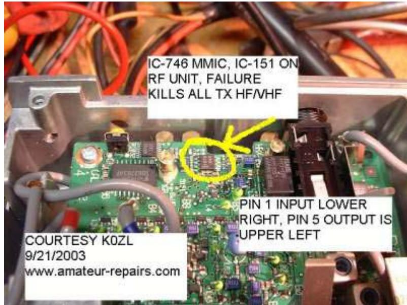
uPD1678, icom number is 1110001890, lists about 10 bucks or less. Changing this chip requires proficiency in surface mount desoldering, and anti-static protection measures.
