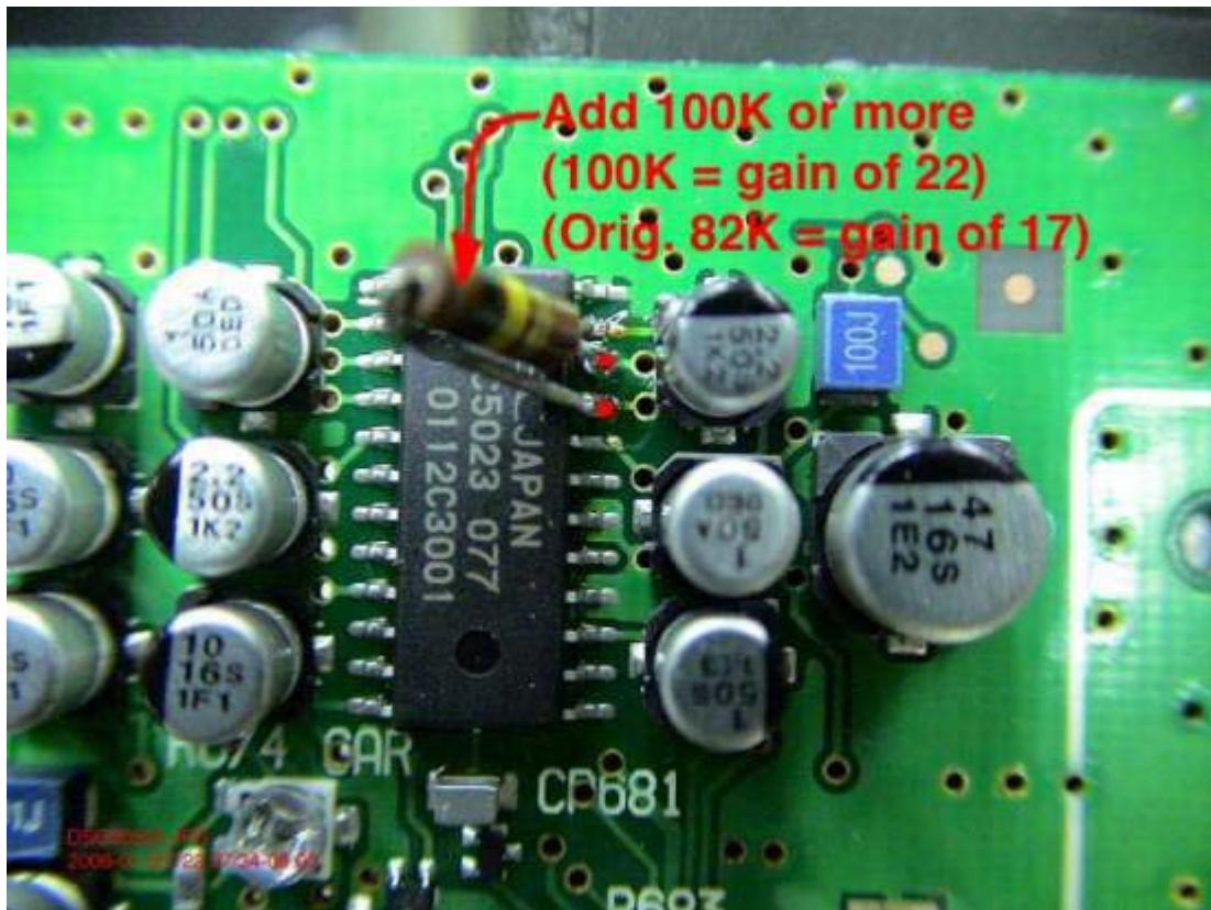
Above: The completed modification; I added a 100K resistor, as shown. Please note that one could put in a potentiometer, but if this is attempted, I would suggest that a 56K resistor be added in series, just to insure that the feedback path does not get too LOW. (A 200 to 300K total value would be more than enough!)
