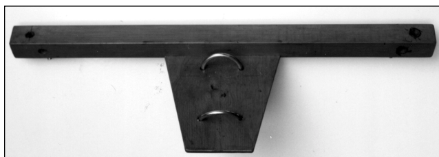
Fig 21 —Photo of the two-element quad's boom, with the plywood boom-to-mast bracket secured with wood screws and glue.
