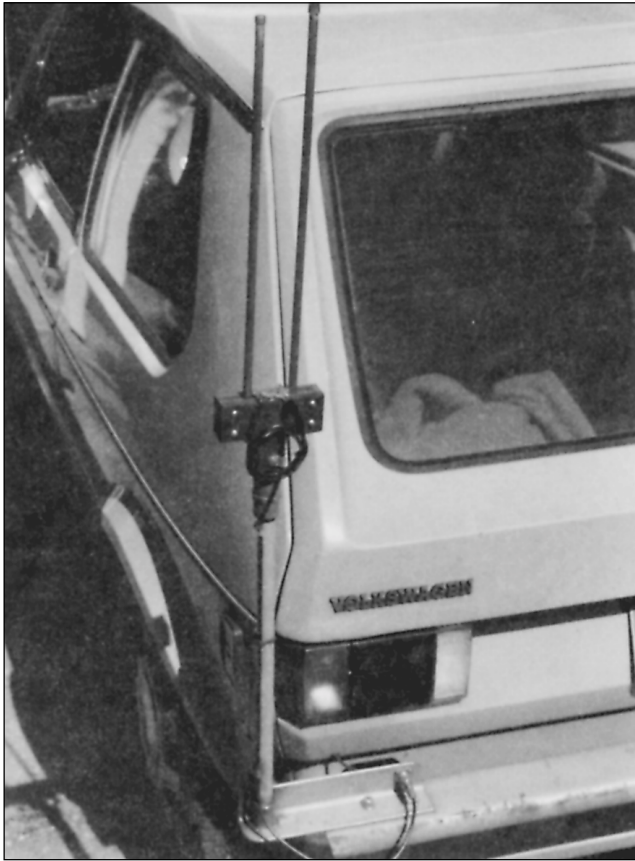
Fig 37—The J antenna, ready for use. Note the bakelite insulator and the method of feed. Tie wraps are used to attach the balun to the mounting block and to hold the coax to the support pipe. Clamps made of flashing copper are used to connect the balun to the J antenna just above the insulating block. The ends of the balun should be weatherproofed.
