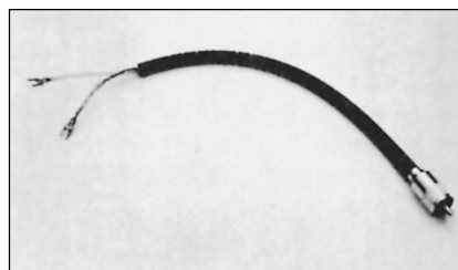
Fig 30—At A, an RF choke formed by coiling the feed line at the point of connection to the antenna. The inductance of the choke isolates the antenna from the remainder of the feed line. See Table 3 for winding data. At B, a bead balun consisting of 50 Amidon no. FB-73-2401 ferrite beads over a length of RG-58A coax. See text for details.
