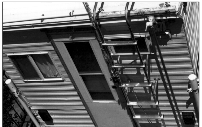
Fig 13 —Photo showing the back of the camper, with the antenna in the lowered position, parallel to the ladder. The “Outback” standby mobile antenna is shown clamped to the left side of the ladder.
