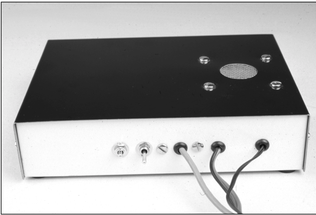
Fig 43—The rear panel of the DF unit supports the two DPDT PHASE toggle switches. Grommets in the panel holes allow abrasion-free passage of the antenna, dc-power and audio cables. The dc power cord is outfitted with an inline fuse holder and a male Jones plug. A six-pin female Molex connector (five pins are used) feeds the four antennas. The audio-input cable is terminated in a 1/8-inch diameter male plug.
