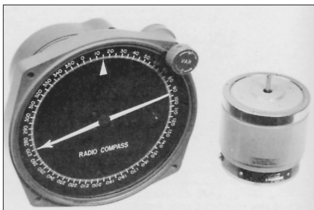
Fig 10—The MN-98 Canadian radio compass and Sperry R5663642 synchro transmitter. Note the small knob at the upper right-hand corner of the indicator face. This can be used to calibrate the system without making any changes at the antenna end. By turning this knob, you can rotate the degree markings around the outside of the dial face so that any desired heading can be placed in line with the pointer.
