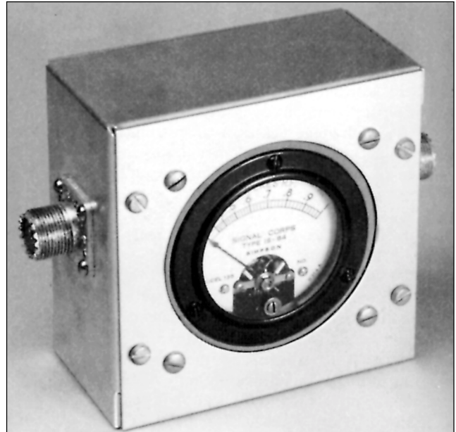
Fig 2—A convenient method of mounting an RF ammeter for use in a coaxial line. This is a metal-case instrument mounted on a thin bakelite panel. The cutout in the metal clears the edge of the meter by about 1/8 inch.
