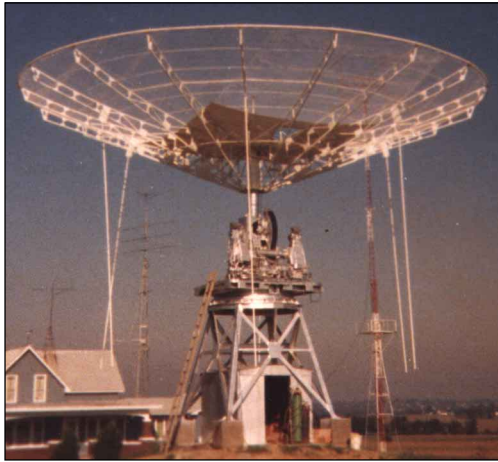
Fig 2 —The gun mount of Fig 1 with its “warhead” attached—a home-made 42-foot parabolic dish. This is part of the arsenal of Ken Kucera, KA0Y.
